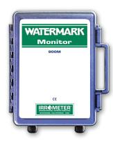
The **900M Monitor** is a battery operated data-logger, that automatically reads up to eight sensors. Users can view readings on the screen, download data to a laptop, or use our Data Shuttle to transport the information to a computer. The 900M Monitor accepts WATERMARK soil moisture sensors, soil and air temperature sensors, switch closure sensors, rain gauge, and IRROMETER RSUs. See Monitor Packages for sensor combination options.
